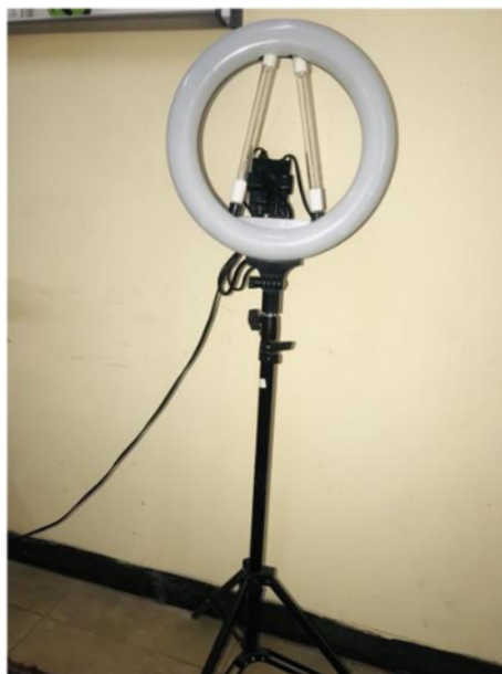
Figure (3.8): 2 UV Leds 254 Nm (Kontec-China) With The Stand.
