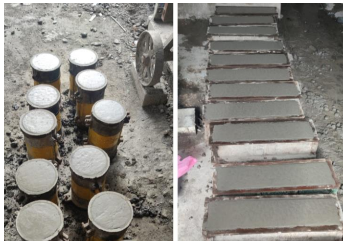
Figure 5. The results of the concrete mixture that has been put into the cylinder and block molds.
