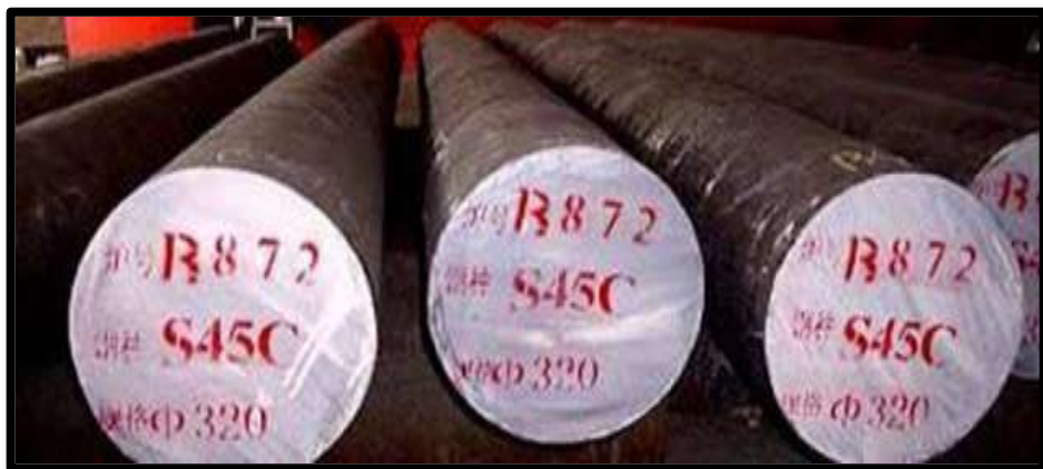
Figure 2. Material Casting S45C
