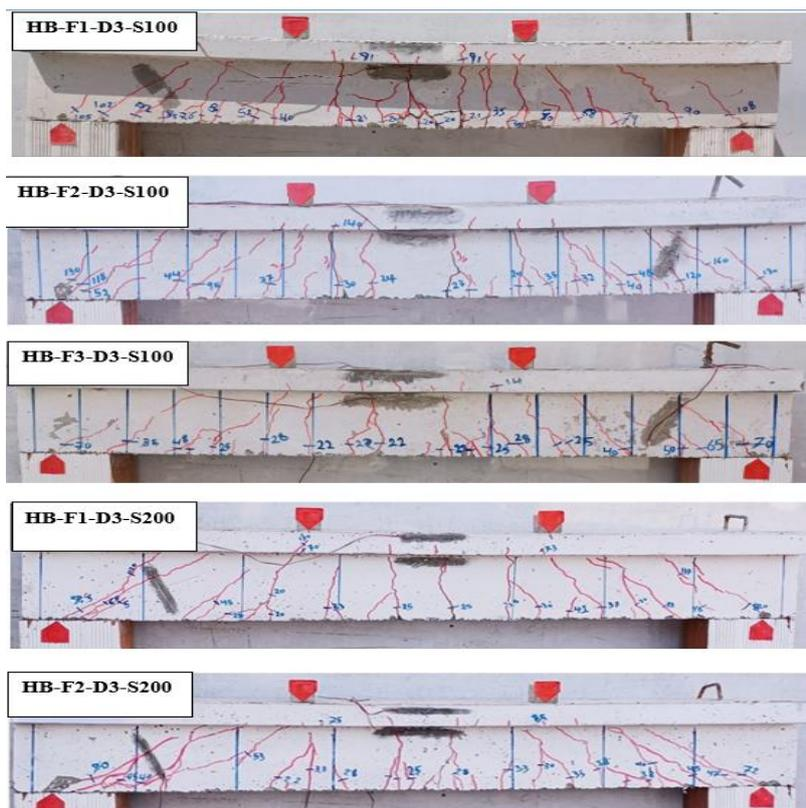
**Figure 6.** Beams after testing.
