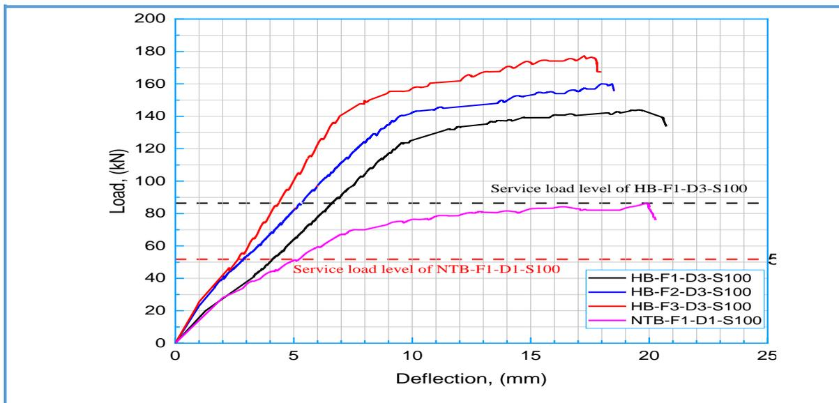
Figure 8. Effect of concrete grade on load-deflection response.
