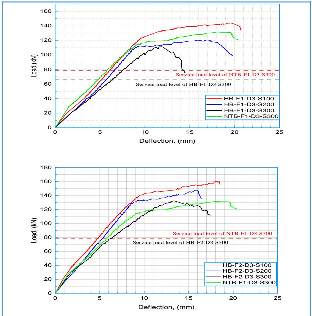
Figure 10. effect of Stirrups spacing on load-deflection behavior.
