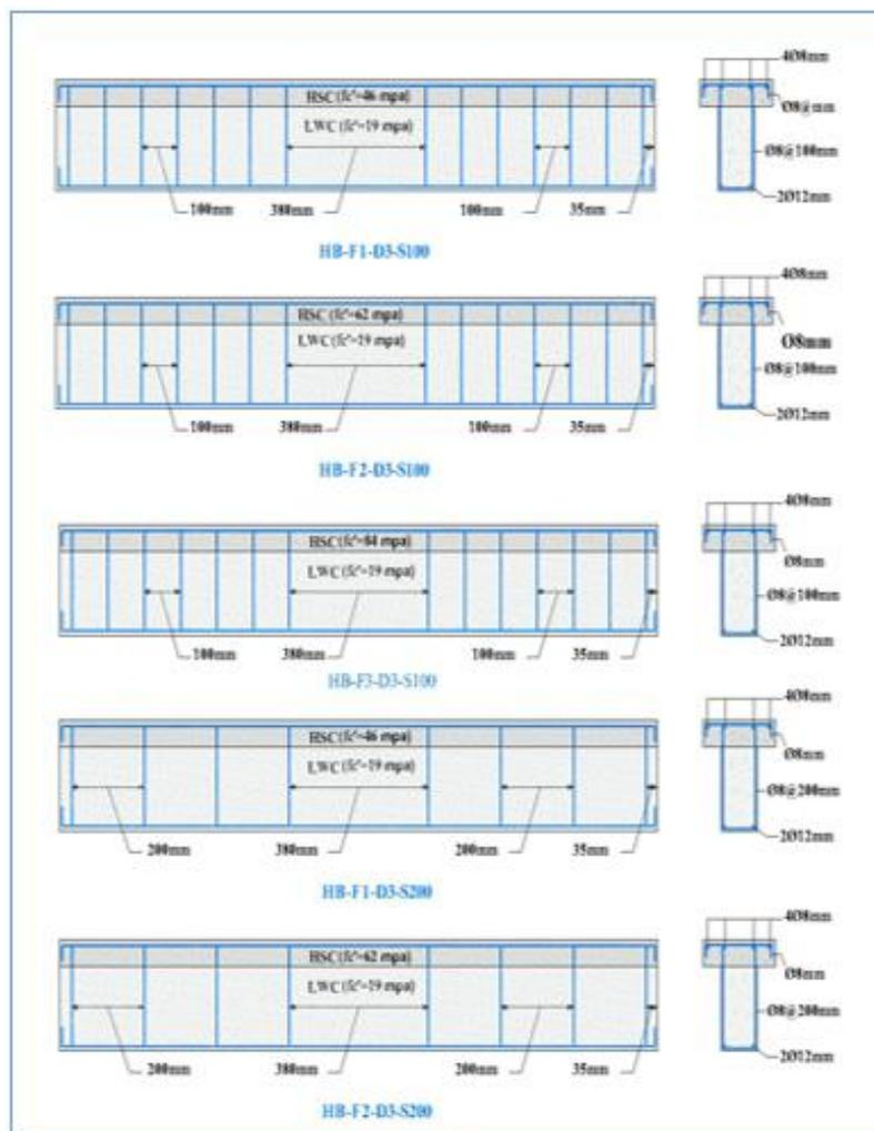
Figure 2. Details of the tested beams.
