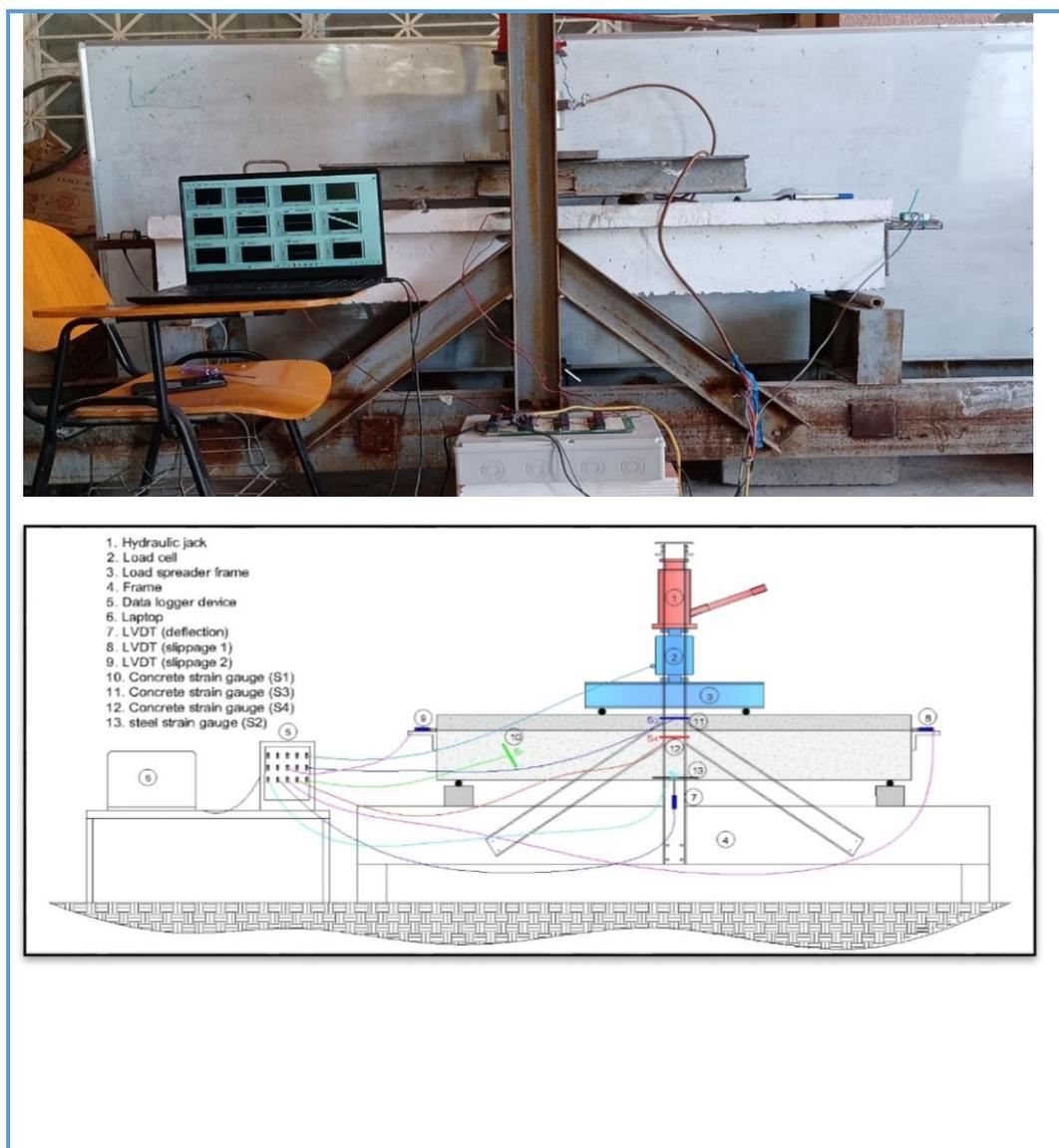
Figure 5. Test setup.
