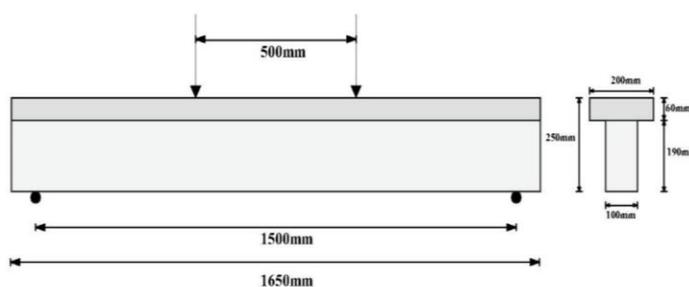
Figure 1. Cross section of the tested beams.
