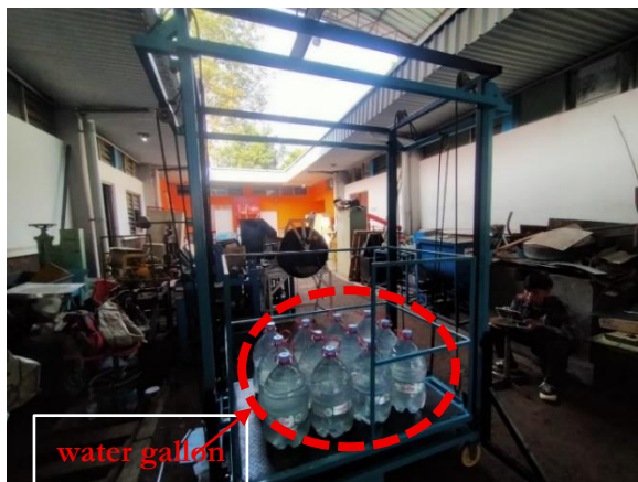
Figure 8. Machine Testing with Load Lifting
