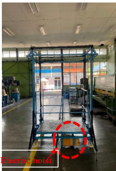
Figure 7. Scaffolding with Electric Hoist Drive
