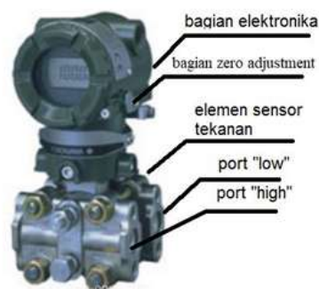
Figure 3. Parts of a Differential Pressure Flow Transmitter.
