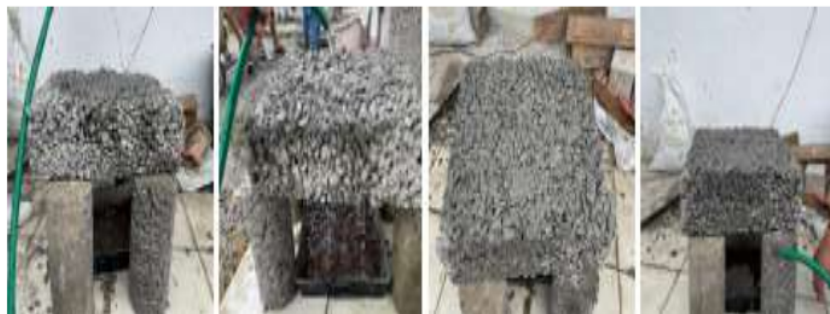
Figure 4.4 water-cement ratio and permeability
