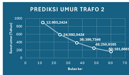
Figure 5. Graphic of Predicted Aging of Traction Transformer 2
