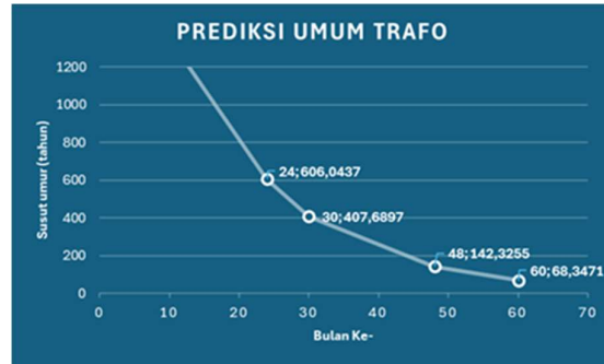
Figure 5. Graphic of Predicted Aging of Traction Transformer 1
