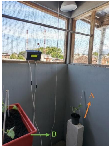
Figure 3. Experimental Setup of the Iot-Based Automatic Lighting System on Melon Plants.
