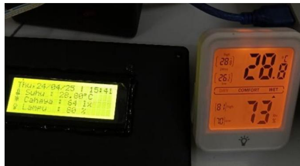
Figure 5. DHT21 Calibration Result.
