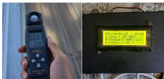
Figure 4. BH1750 Calibration Result.
