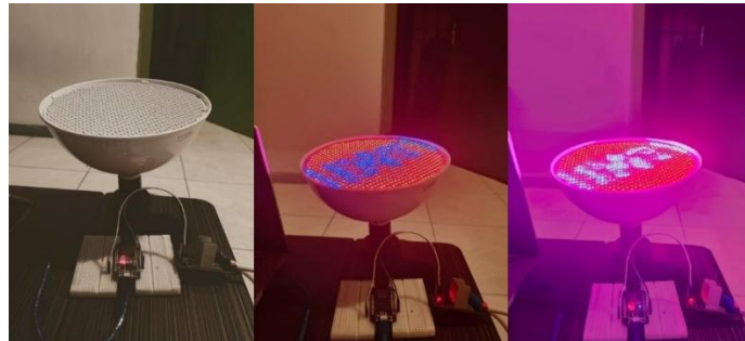
Figure 6. AC Light Dimmer Testing on LED Grow Light.
